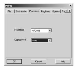
5 Click the **Options** tab. Make sure that the **Reset Target** and **Load Application Image** check boxes are selected, as shown.
